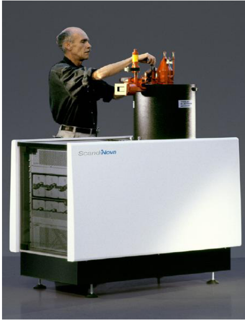
Fig. 10. The 7.5MW klystron is powered by a solid state modulator commercialized by ScandiNova Systems AB (Uppsala). LIBO employs 10 modulator/klystron systems.
